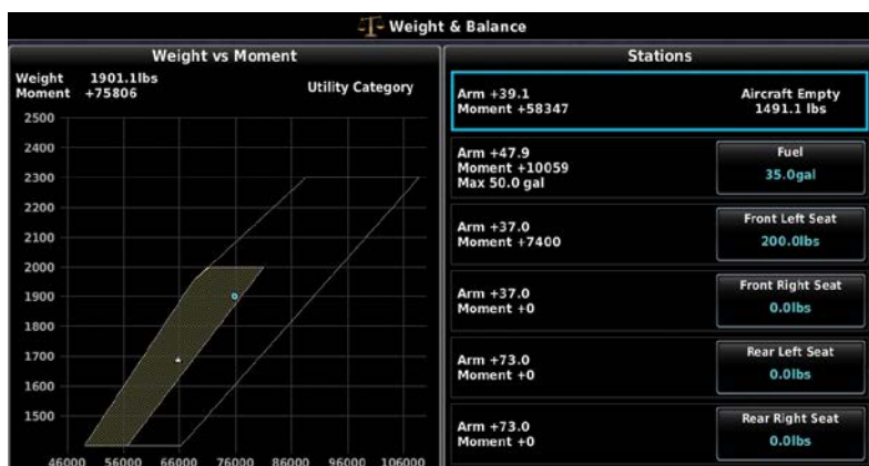
Weight and Balance Page - Weight vs Moment
