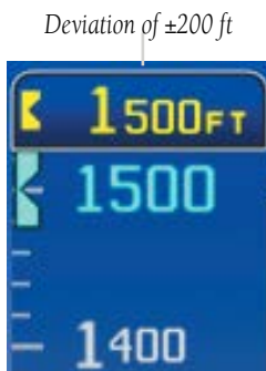
Altitude Alerting Visual Annunciation
