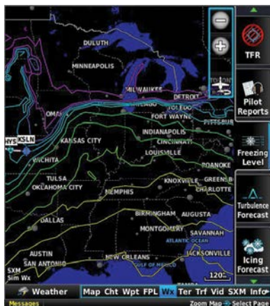
Freezing Level Data
