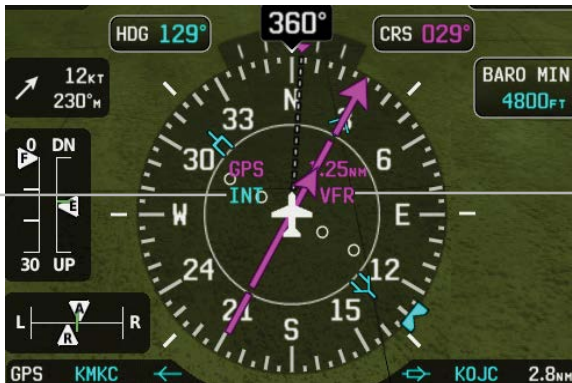
Intentional Pilot Selection of Internal GPS Navigation
