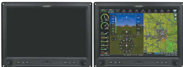
G3X Touch Full-Screen Reversionary Mode (Failed PFD)
