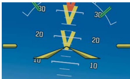
ESP Engaged (Nose-High)
