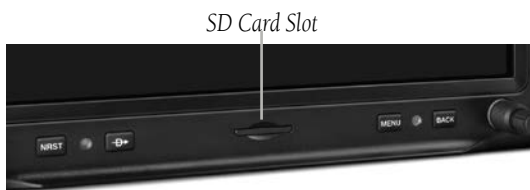
SD Card Slot - GDU 46X (10.6 inch)
