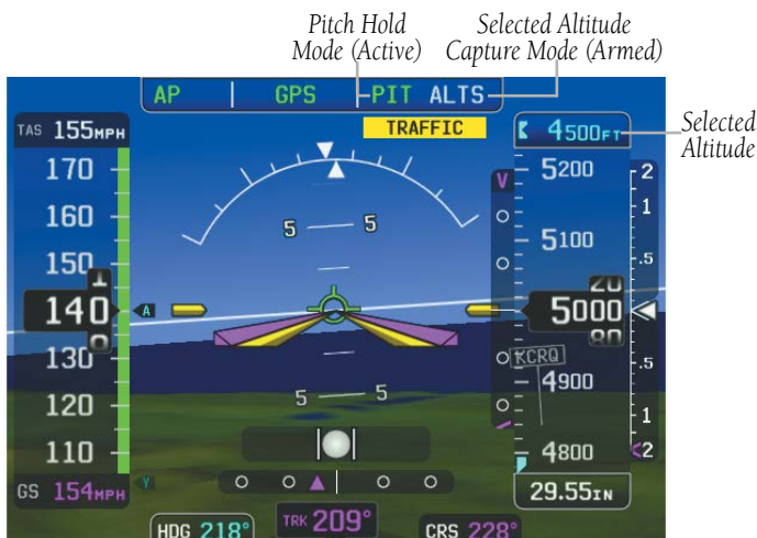
Pitch Hold & Selected Altitude Capture Modes
