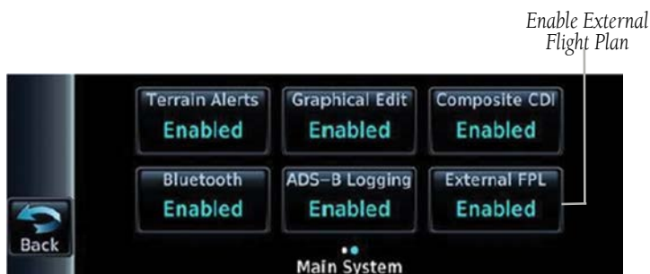
External Flight Plan Enabled (Configuration Mode)
