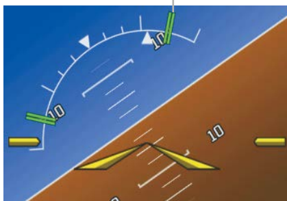
Roll Increasing to ESP Engagement
