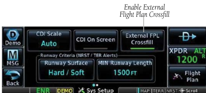
External Flight Plan Crossfill Enabled (Normal Mode)
