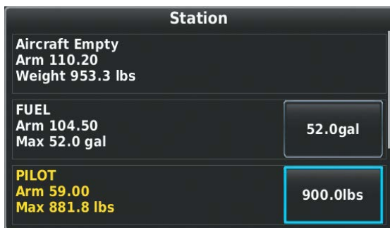
Loading Limit Exceeded
