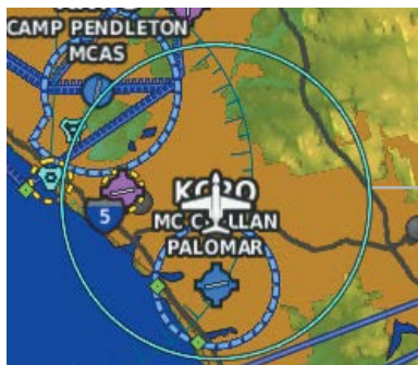
Navigation Map - Glide Range Ring (Ideal Descent Profile - No Wind)
