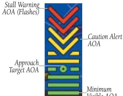
Angle of Attack Display (AOA)
