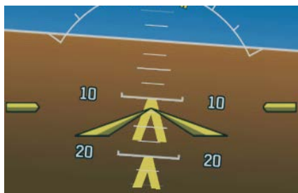
ESP Engaged (Nose-Low)
