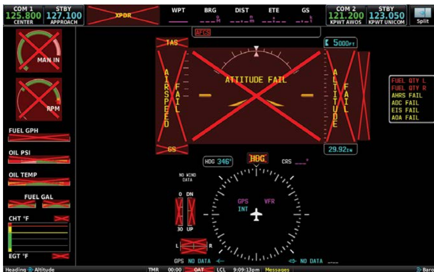
G3X Touch System Failure Annunciations
