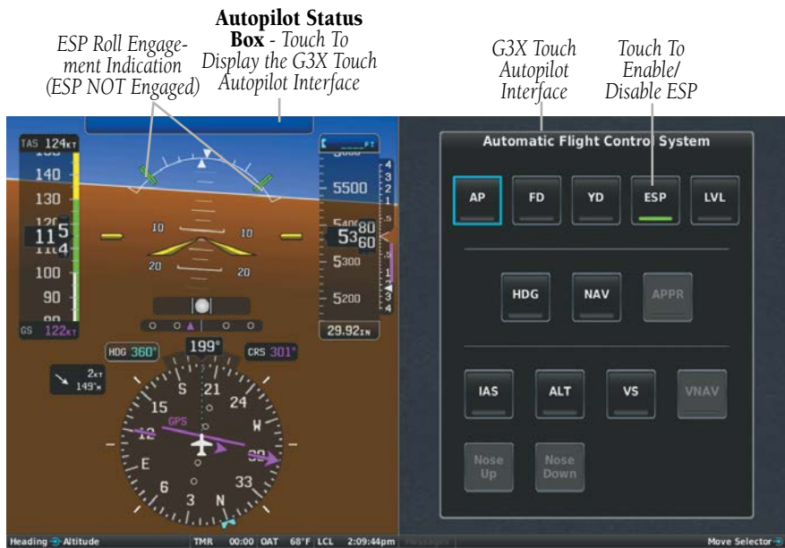
AFCS (ESP Enabled)
