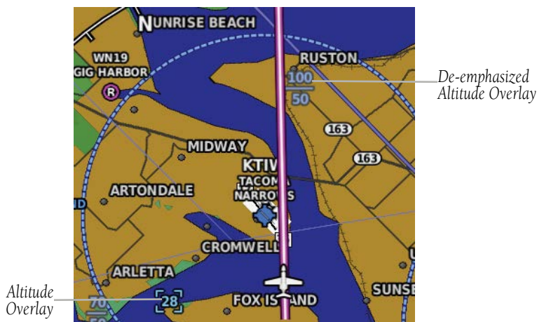
Smart Airspace™ with Altitude Overlays
